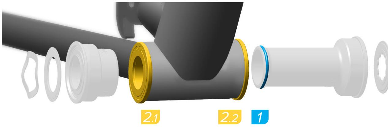
Use a headset press or bottom bracket bearing press tool to install the drive side bearing cup into the frame according to the tool manufacturer's instructions. Repeat the installation with the non-drive side bearing cup.
