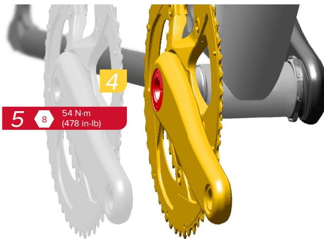
Use a torque wrench with an 8 mm hex bit socket to tighten the crank arm bolt to 54 N·m (478 in-lb). Use a mallet to tap the drive side crank arm until it is fully seated.
