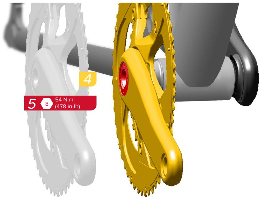
Use a torque wrench with an 8 mm hex bit socket to tighten the crank arm bolt to 54 N·m (478 in-lb). Use a mallet to tap the drive side crank arm until it is fully seated.
