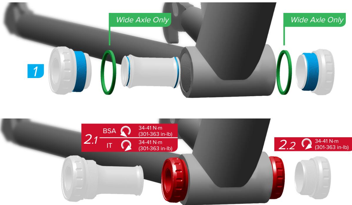
Use a GXP bottom bracket tool to tighten the cups into the frames.
